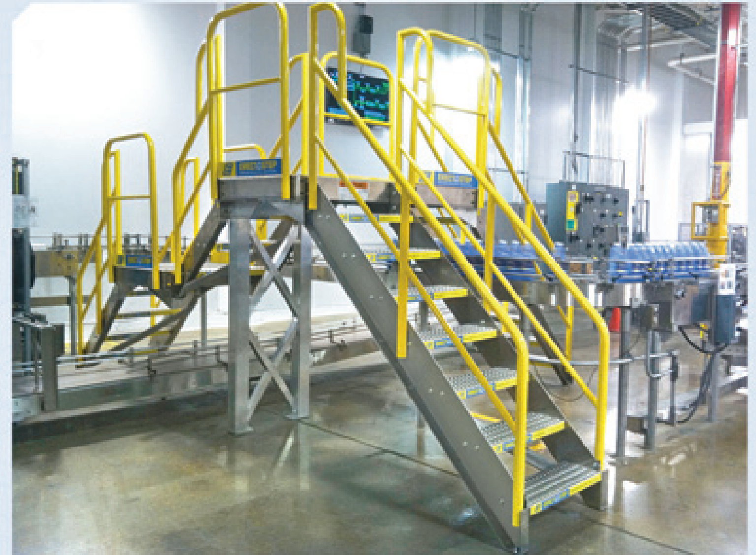
The components from this crossover can be re-purposed as the plant grows.
